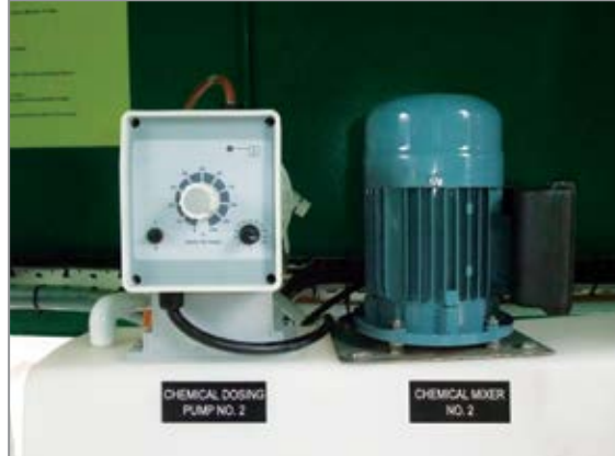
2 Automatic Chemical Mixing & Dosing System
